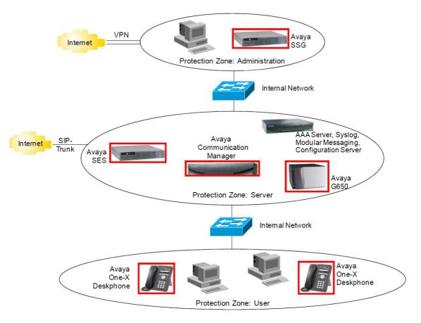
Figure 1: Structure of the VoIP System
