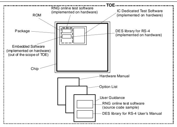
Figure 1-1: Configuration of the TOE
