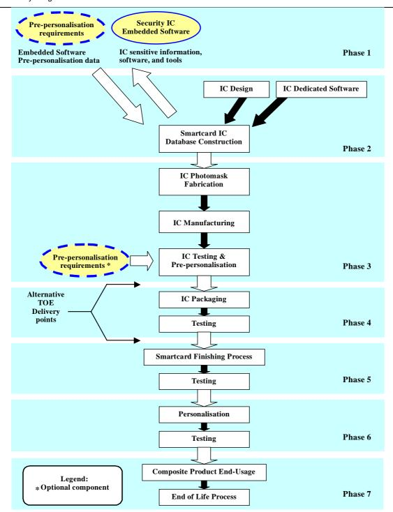
Figure 1-3: Design and Manufacturing Lifecycle
