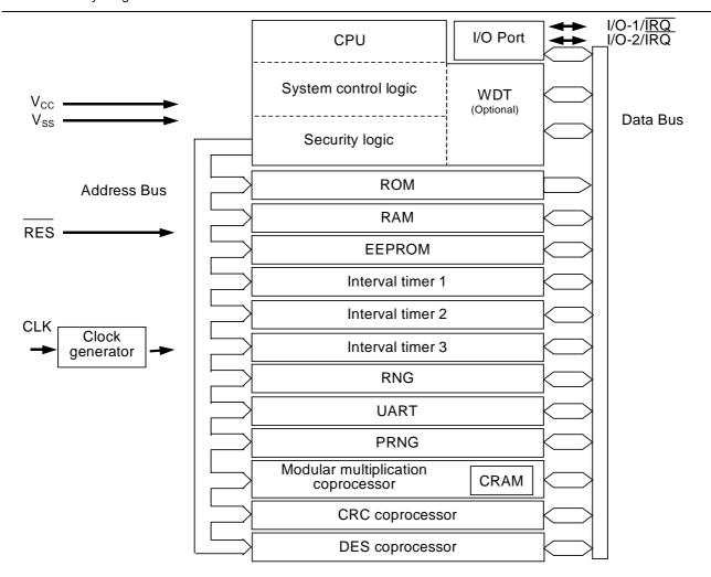
Figure 1-2: Internal Block Diagram of the TOE
