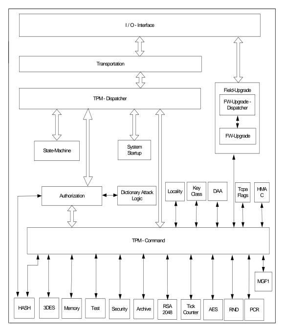
Figure 2: Firmware block diagram of the SLB9635TT1.2
