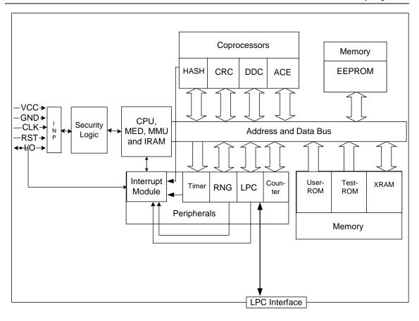
Figure 1: Block diagram of the SLB9635TT1.2
