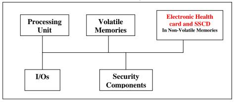
Figure 1 – Smart card IC with Embedded Software
