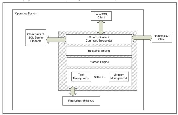
Figure 1 - TOE structure
