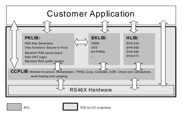
Figure 1-2: RCL (TOE Software), TOE Hardware and Customer Application
