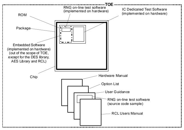
Figure 1-1: Configuration of the TOE
