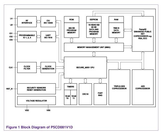
The IC Dedicated Software is a composition of IC Dedicated Test Software and IC Dedicated Support Software. The IC Dedicated Software is part of the ROM memory. All other software is called Security IC Embedded Software and is not part of the TOE. In the following Table 1 lists the TOE components.
