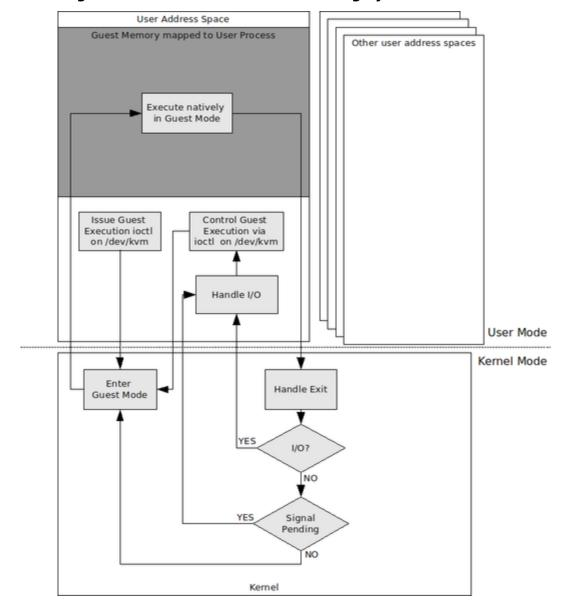
Figure 1: KVM virtual machine handling by the Linux kernel
