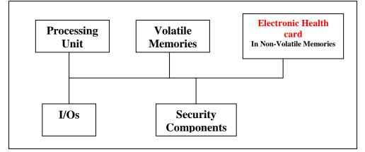
**Figure 1 – Smart card IC with Embedded Software**
