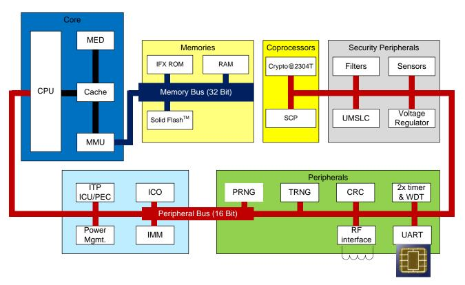
Figure 1: Block diagram of the TOE
