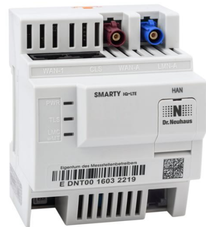
Figure 3: SMARTY IQ-LTE casing and external interfaces
