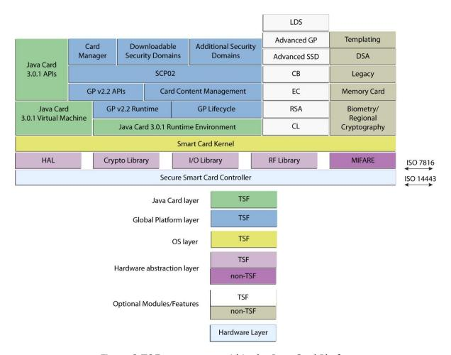
Figure 2 TOE components within the Java Card Platform
