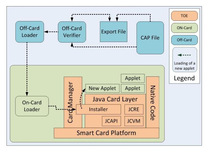
Figure 3 Java Card Platform and applet installation environment
