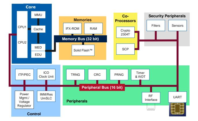
Figure 1: Simplified block diagram of the TOE
