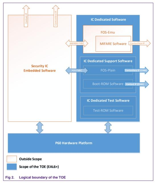
Fig 2 also shows that the FOS-Emu including the MIFARE Software is not part of the TOE.
