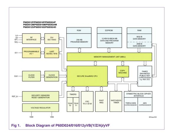
The TOE consists of the IC hardware platform and Security IC Dedicated Software as composed of Security IC Dedicated Test Software and Security IC Dedicated Support Software. The Security IC Dedicated Test Software contains the Test-ROM Software; the Security IC Dedicated Support Software contains the Boot-ROM Software and the Firmware Operating System.All other software is called Security IC Embedded Software. The Security IC Embedded Software is not part of the TOE.
