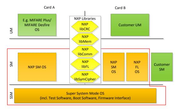
Fig. 1.2: Software Components of the TOE
