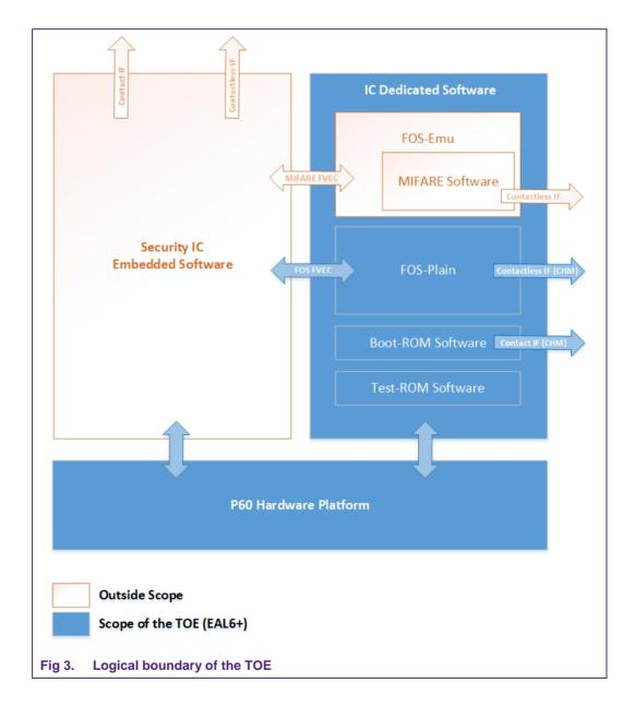
Fig 3 also shows that the FOS-Emu including the MIFARE Software is not part of the TOE.
