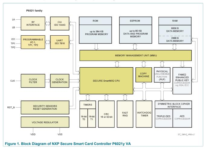
The P6021y VA contains the IC hardware platform and the IC Dedicated Software which is composed of IC Dedicated Test Software and IC Dedicated Support Software. All other software is called Security IC Embedded Software. The Security IC Embedded Software is not part of the P6021y VA.
