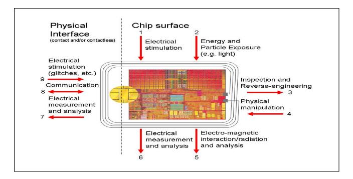
Figure 7: Interactions between the TOE and its outer world
