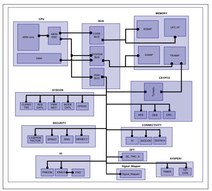
Figure 1: S3FV9VH Block Diagram
