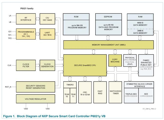
The P6021P VB contains the IC hardware platform and the IC Dedicated Software which is composed of IC Dedicated Test Software and IC Dedicated Support Software. All other software is called Security IC Embedded Software. The Security IC Embedded Software is not part of the P6021P VB.
