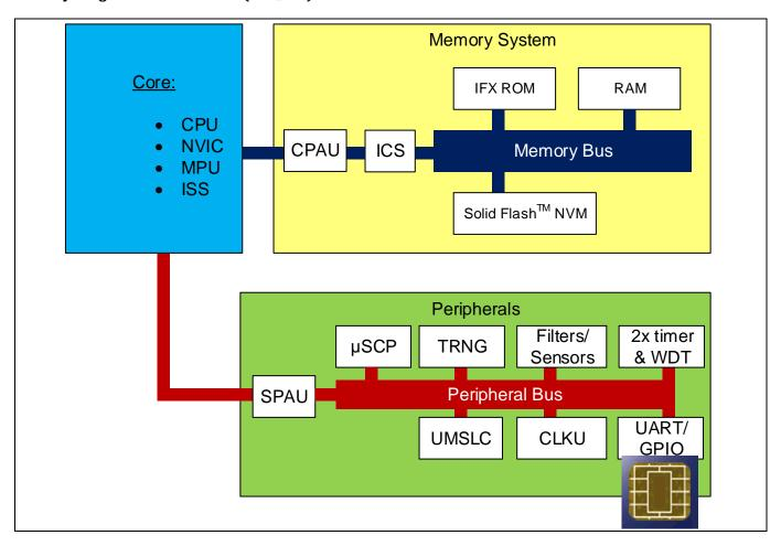
The TOE hardware consists of a core, a memory system and peripherals.
