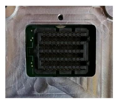
Figure 7: The KM Mezzanine connector
