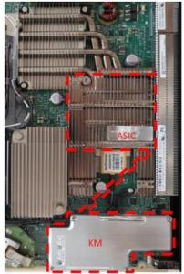
Figure 5: The TOE on the Ciena 6500 Flex3 WaveLogic 3e OCLD Circuit Pack (Bottom & Top View)
