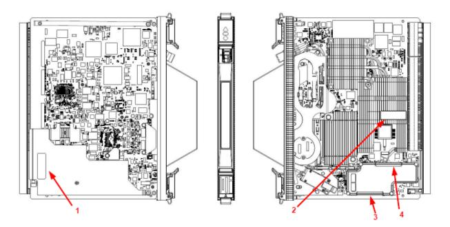
Figure 6: Tamper-Evident Label Locations
