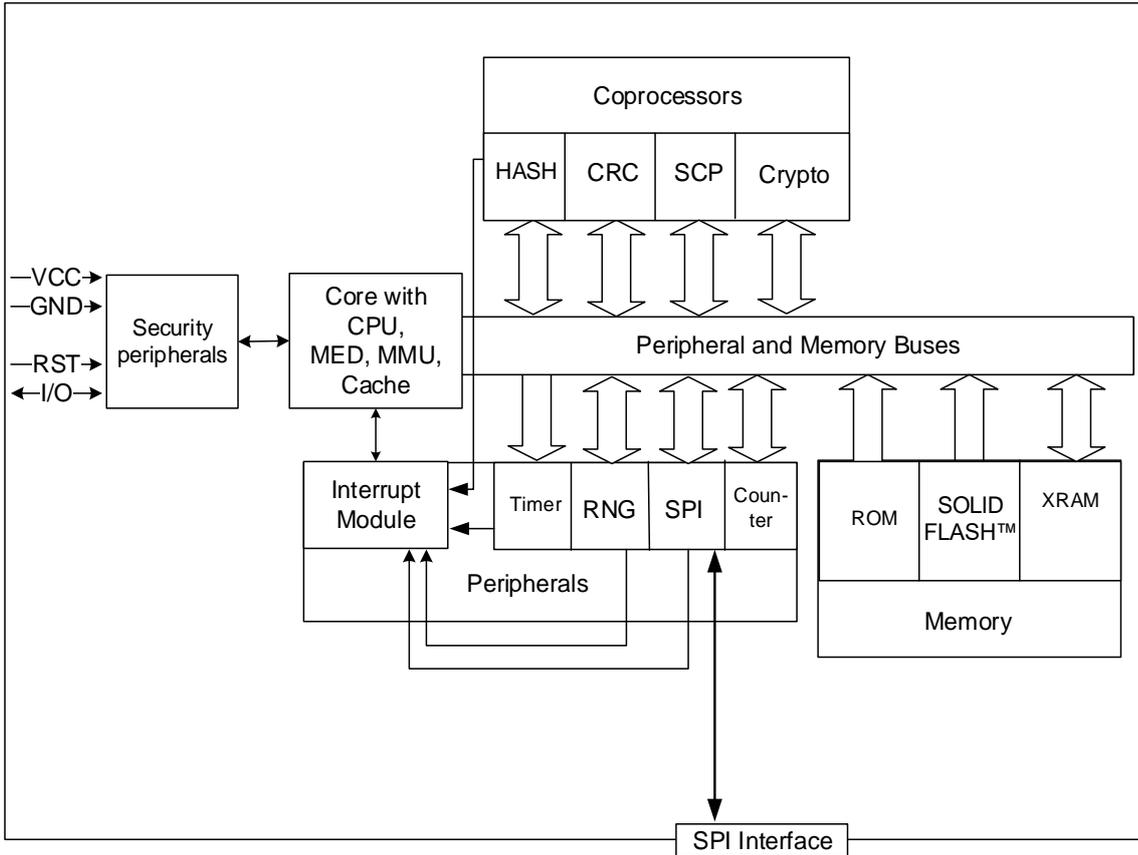
Figure 1: Block diagram of the SLI9670\_2.0
