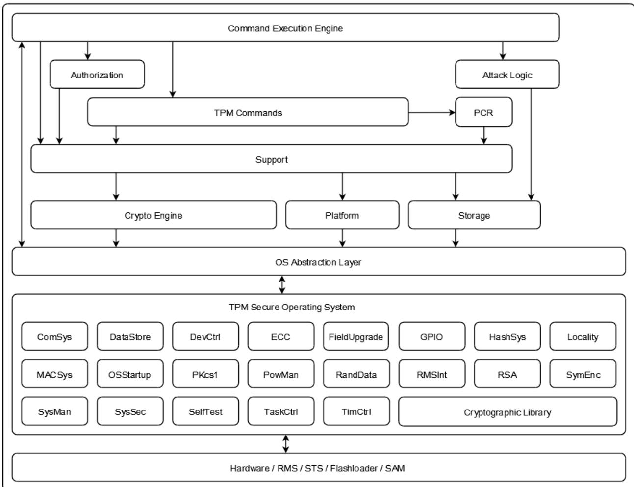
Figure 2: Firmware block diagram of the SLI9670\_2.0
