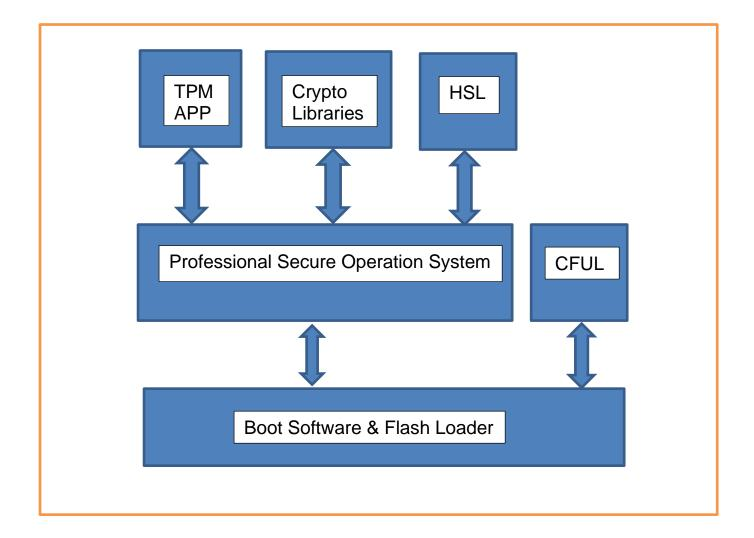
Figure 2: Firmware block diagram of the SLB9672\_2.0
