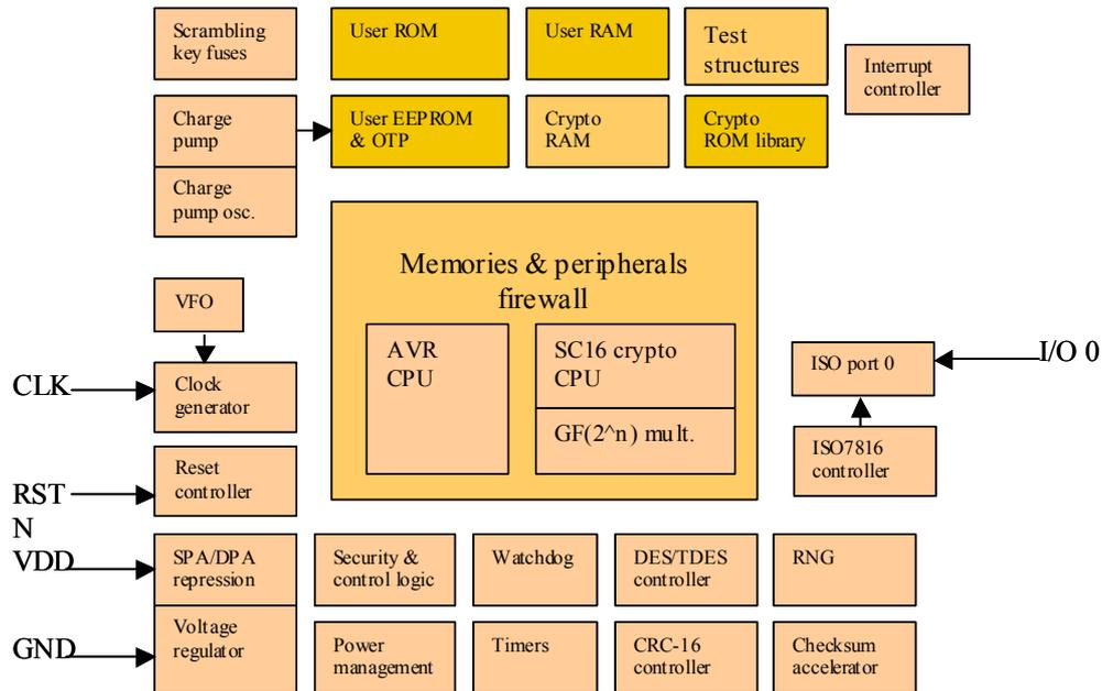
Figure 1 - micro-circuit ATMEL AT90SC19272RC
