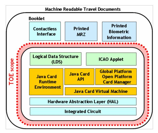
The TOE is defined to comprise the chip and the complete operating system and application. Note, the inlay holding the chip as well as the antenna and the booklet (holding the printed MRZ) are needed to represent a complete MRTD, nevertheless these parts are not inevitable for the secure operation of the TOE.
