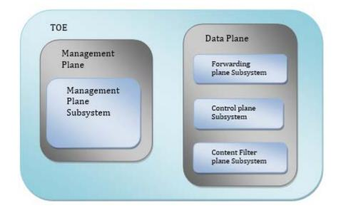
The TOE software is divided into two different planes: Management Plane (MP) a Data Plane (DP). MP is composed by only one subsystem called Management plane Subsystem. DP is composed by three subsystems called Forwarding plane Subsystem, Control plane Subsystem, and Content Filter Subsystem.
