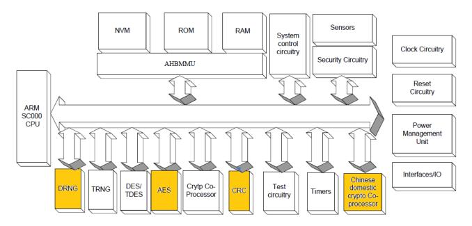
The hardware of the TOE has the following components:
