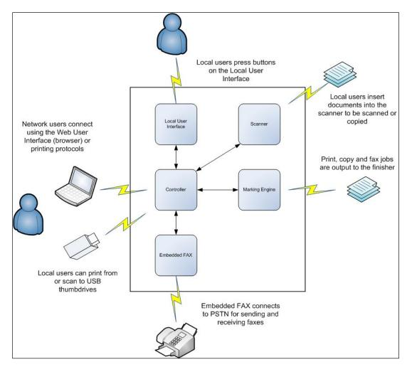
Figure 1: Architectural Diagram of the TOE
