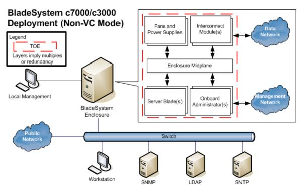
Figure 8 - Physical TOE Boundary - Non-VC Mode
