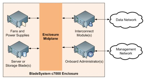
Figure 6 - Non-VC Mode Deployment Configuration of the TOE
