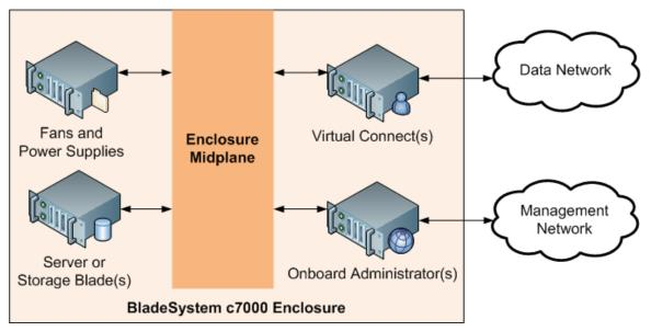
Figure 5 - VC Mode Deployment Configuration of the TOE
