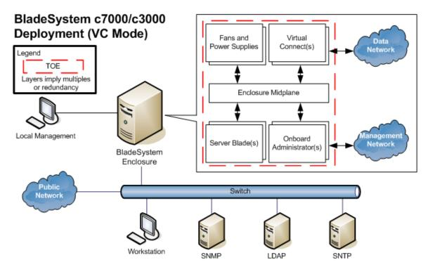
Figure 7 - Physical TOE Boundary - VC Mode
