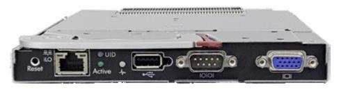
Figure 2 - HP BladeSystem OA Module (Example)
