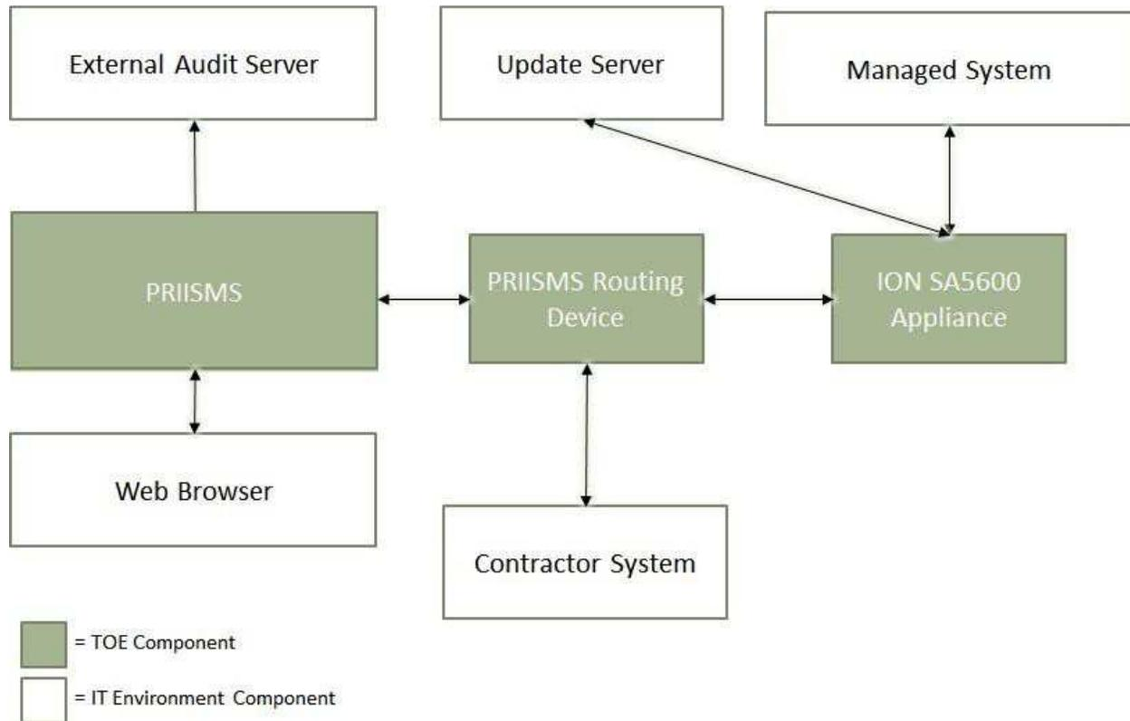
Figure 1 –Deployed TOE
