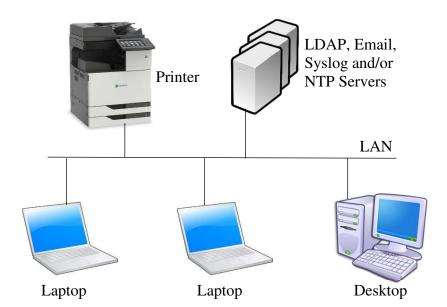
Figure 1 - Representative TOE Deployment
