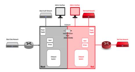
Figure 1: TOE Architecture
