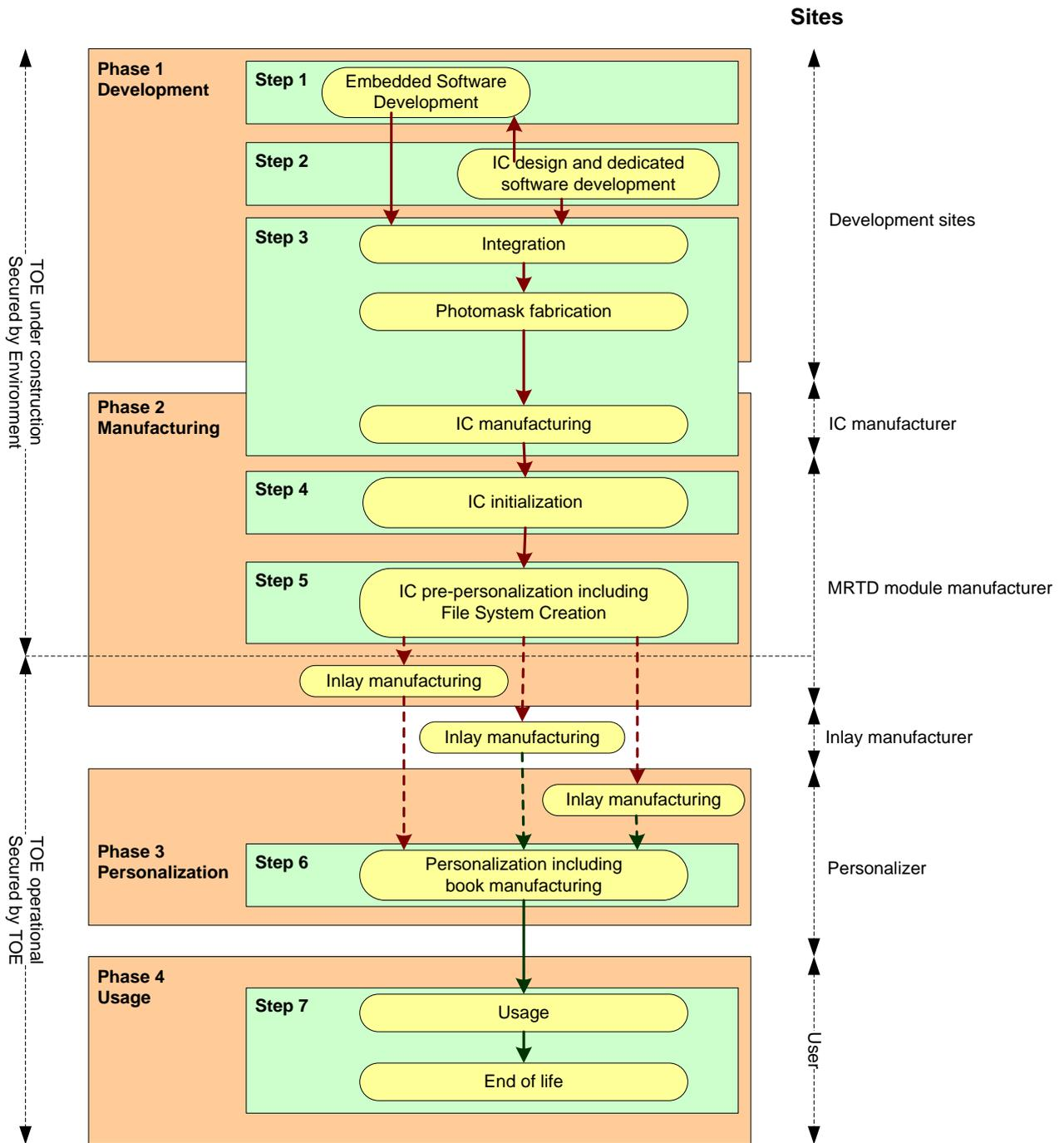
Figure 2: LC1: Init on module at Gemalto site
