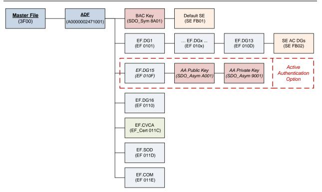
Figure 2 - Typical BAC LDS for IDPass
