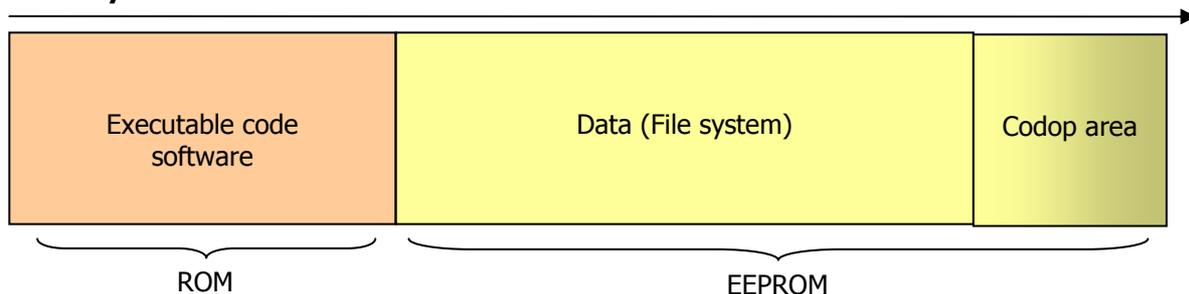
**Figure 2** Memory mapping of the TOE
