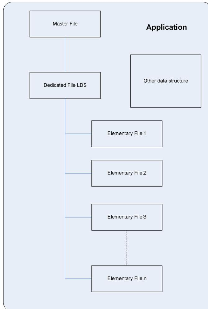
**Figure 3 : Structure of the file system**
