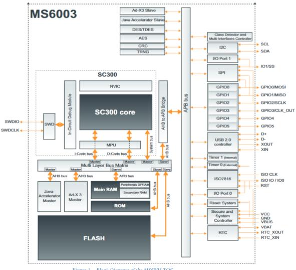
Figure 1 Block Diagram of the MS6003 TOE
