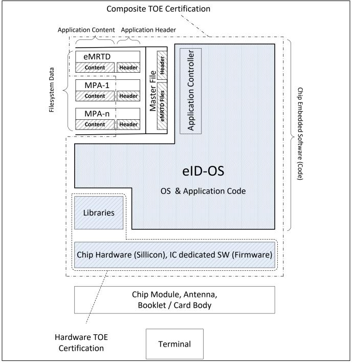
Figure 1 TOE block diagram
