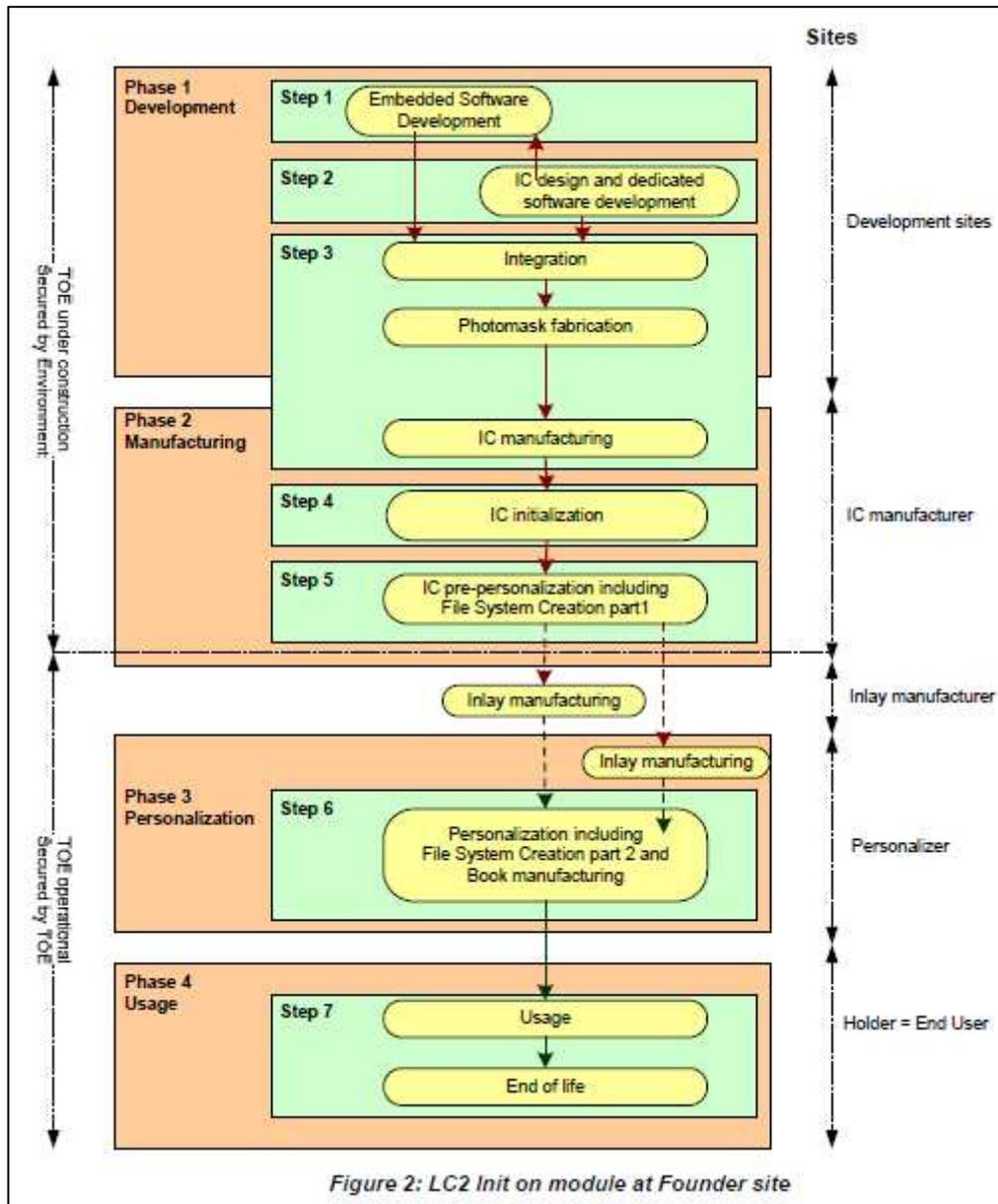
Figure 2: LC2 Init on module at Founder site
