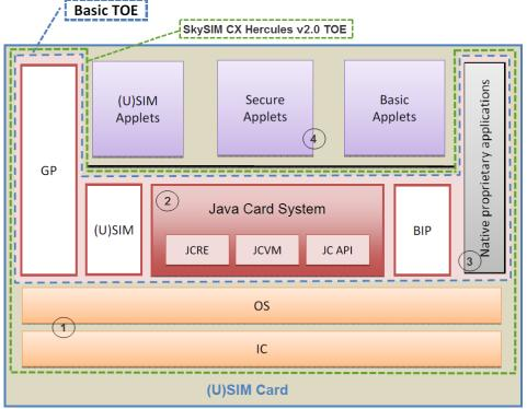
Figure 1 (U)SIM PP Basic TOE and the SkySIM CX Hercules v2.0 TOE
