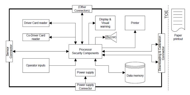
Figure 1: Block Diagram of the TOE
