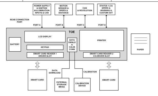
Figure 3: TOE Operational Environment
