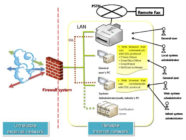
Figure 1: Operating Environment of the TOE
