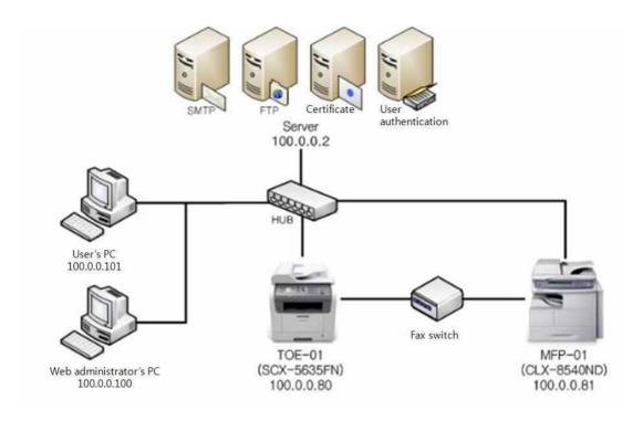
[Figure 3] Evaluator test configuration
