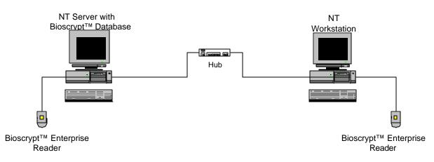
A typical Bioscrypt<sup>TM</sup> Enterprise set-up for a Microsoft Windows domain is shown in Figure 1.
