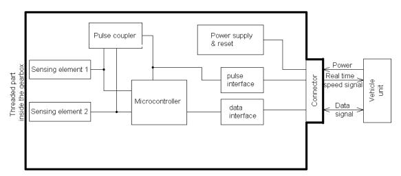
Figure 1, TOE hardware structure
