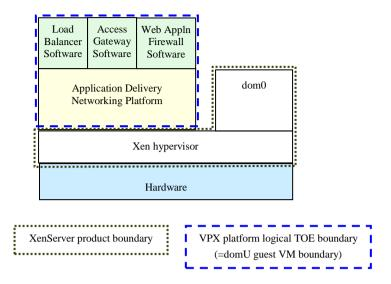
Figure 3: VPX Platform TOE detail
