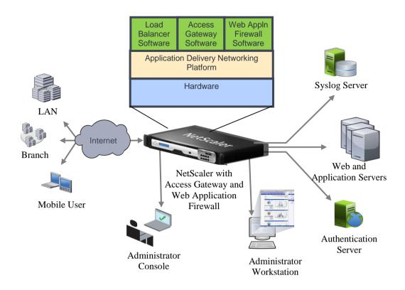
Figure 1: Deployment Configuration of the Product
