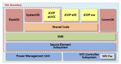
TOE identification provided in the ST identifies the JCOP OS with eUICC functionalities and including Shared Code (with Cryptolib), FlashOS, CommOS, SystemOS, and SMK. There are no known applications loaded pre-issuance or post-issuance for this evaluation.
