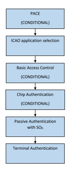
The Chip Authentication step in Figure 3-1 may be skipped if a PACE-CAM authentication has been successfully performed.
