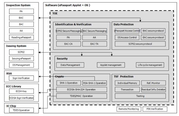
Figure 6 Logical Scope of TOE
