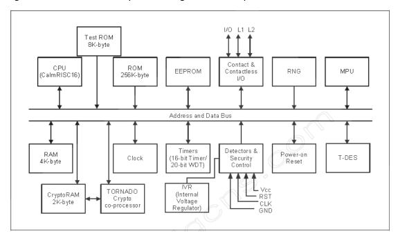
**Figure 3 IC Chip Hardware Composition Diagram**
