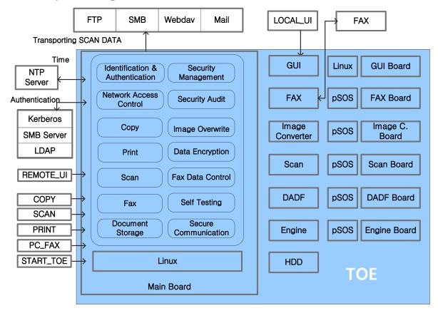
Figure 2: Physical Structure of MFP
