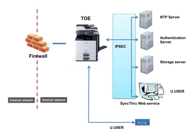
Figure 1: Operational Environment of the TOE
