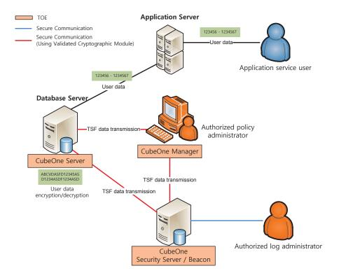
[Figure 1] Operational environment of the TOE (Plug-in type)
